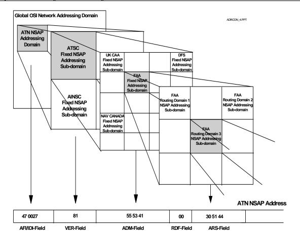
Figure 4-1. Hierarchical Decomposition of Addressing Domains Illustrated for ATN Network Addresses
