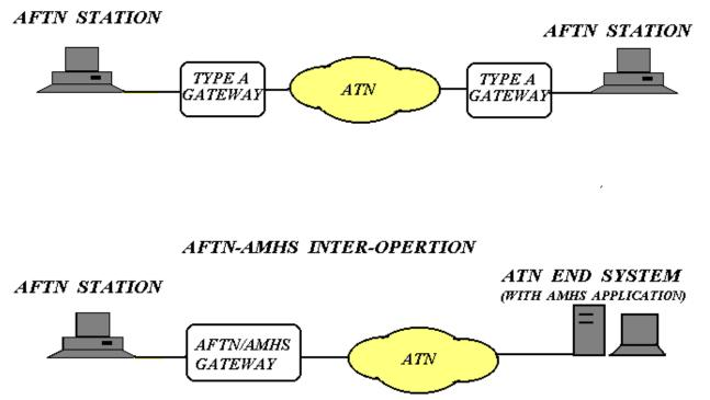
Figure 7-1. AFTN/ATN Gateway System Concept
