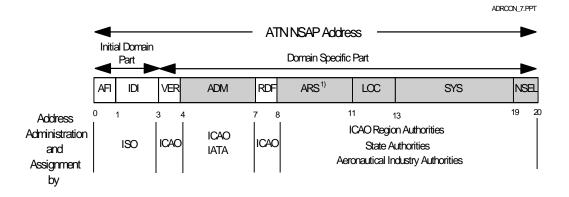
Figure 4-3. ATN NSAP Address Format
