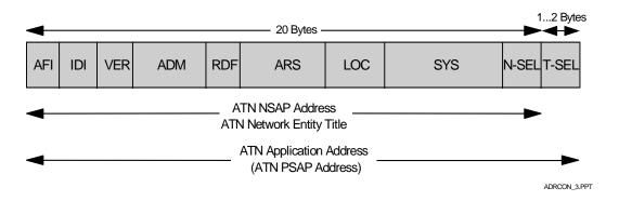
Figure 4-5. ATN Application Address Format for ATN Datalink Applications, AIDC Applications and AFTN/ATN Type A Gateways
