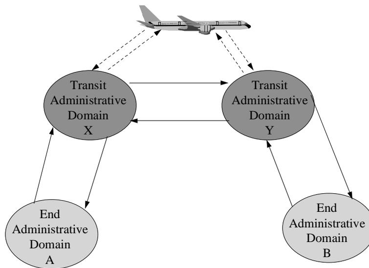
Consider the figure above and assume that an ES in Administrative Domain A is communicating with an ES on board the aircraft. We must consider whether the accounting principles recommended in section 4.2.1 can be applied in an A/G internet communication scenario context.
