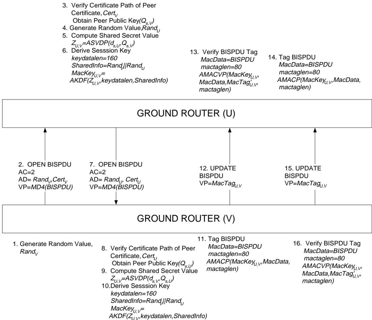
Figure 2 – Ground-Ground Router IDRP Authentication Exchanges
