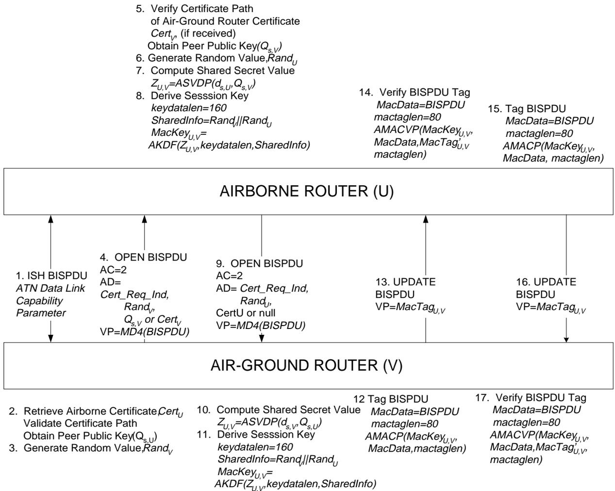
Figure 1 – Airborne and Air-Ground Router IDRP Authentication Exchanges
