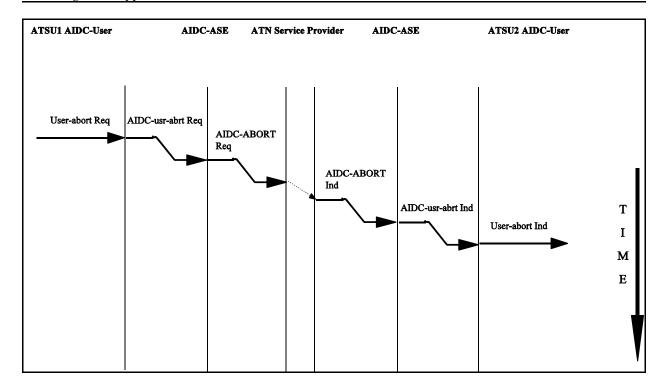
Figure 3.2.10-26: Sequence Diagram for the User-abort service
