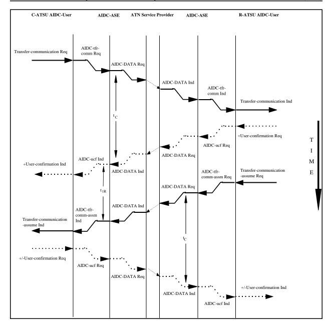
Figure 3.2.10-17: Sequence Diagram showing the invocation of the Transfer-communications service with the invocation of the Transfer-communications-assume service
