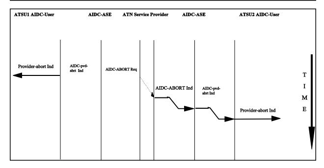
Figure 3.2.10-28: Sequence Diagram showing the service invocation sequence when the AIDC-ASE aborts
