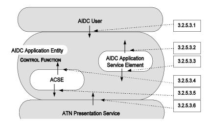
Figure 3.2.5-1: Elements of the AIDC-AE
