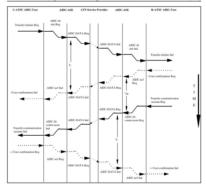
Figure 3.2.10-13: Sequence Diagram showing the invocation of the Transfer-communicationassume service after the Transfer-initiate service
