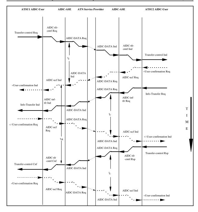
Figure 3.2.10-23: Sequence Diagram showing the invocation of the Info-transfer service in the Transferrring Regime
