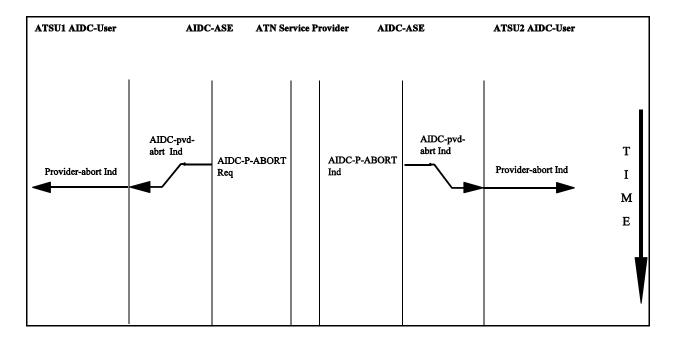
Figure 3.2.10-27: Sequence Diagram showing the invocation of the Provider-abort service invoked by the ATN service provider
