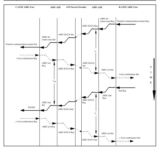
Figure 3.2.10-18: Sequence Diagram showing the end of the AIDC service through the invocation of the End service after the Transfer-communication-assume service
