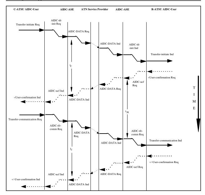
Figure 3.2.10-12: Sequence Diagram showing the invocaton of the Transfer-communication service after the Transfer-initiate service
