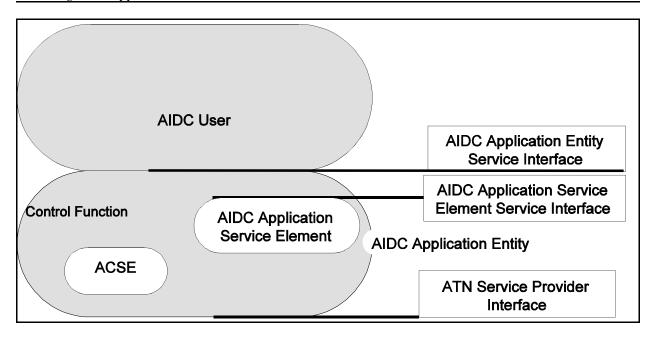
Figure 3.2.1-1: Functional Model of the AIDC Application
