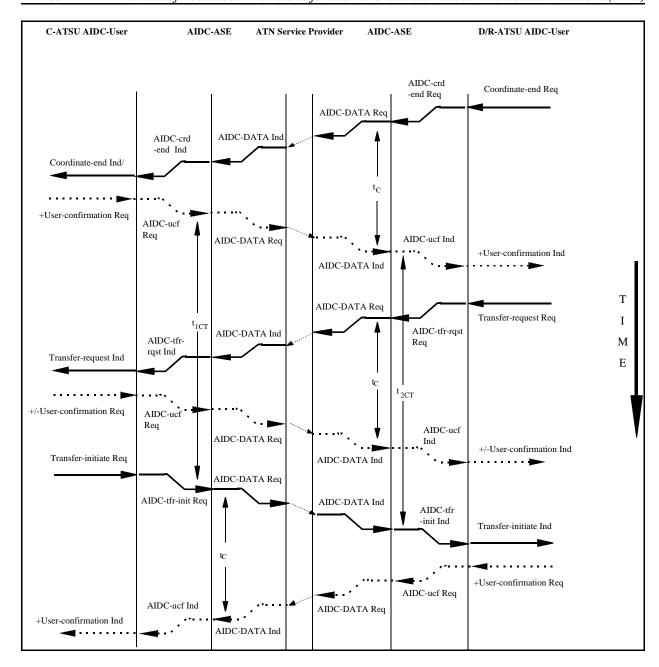
Figure 3.2.10-11: Sequence Diagram showing the invocation of the Transfer-request service
