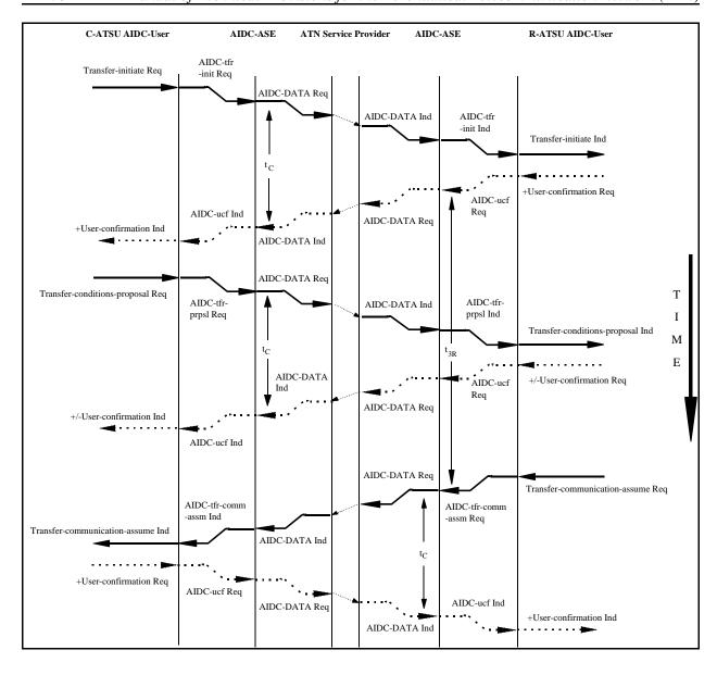
Figure 3.2.10-15: Sequence Diagram showing the invocation of the Transfer-conditions-proposal service, with the predicate P1 false, followed by the invocation of the Transfer-communication-assume service
