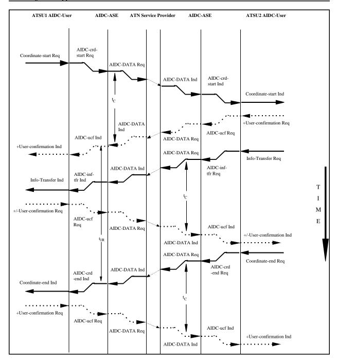
Figure 3.2.10-22: Sequence Diagram showing the invocation of the Info-transfer service in the Coordinating Regime
