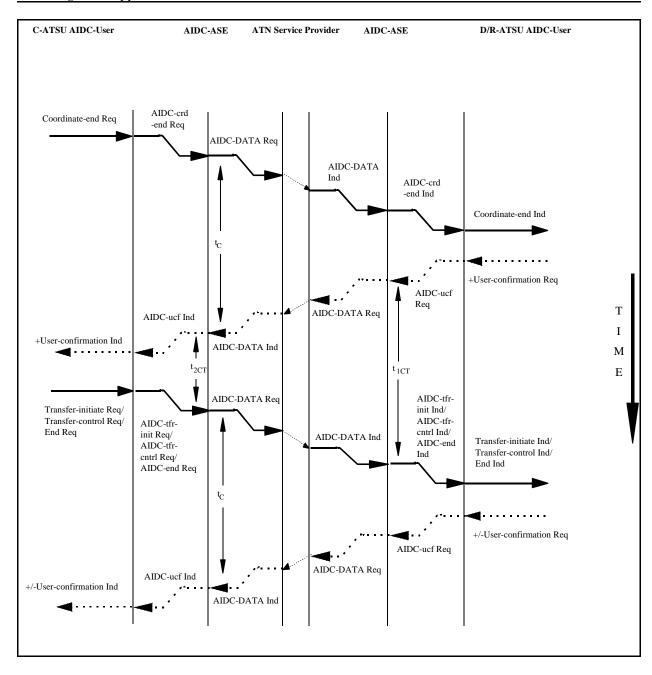
Figure 3.2.10-8: Sequence Diagram showing the start of the Transferring Regime through the invocation of the Transfer-initiate service
