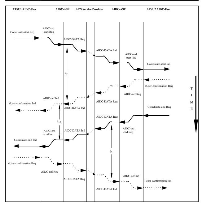
Figure 3.2.10-2: Sequence Diagram showing the entry and exit of the Coordination Regime through the invocation of the Coordinate-start Service and the Cordinate-end Service respectively
