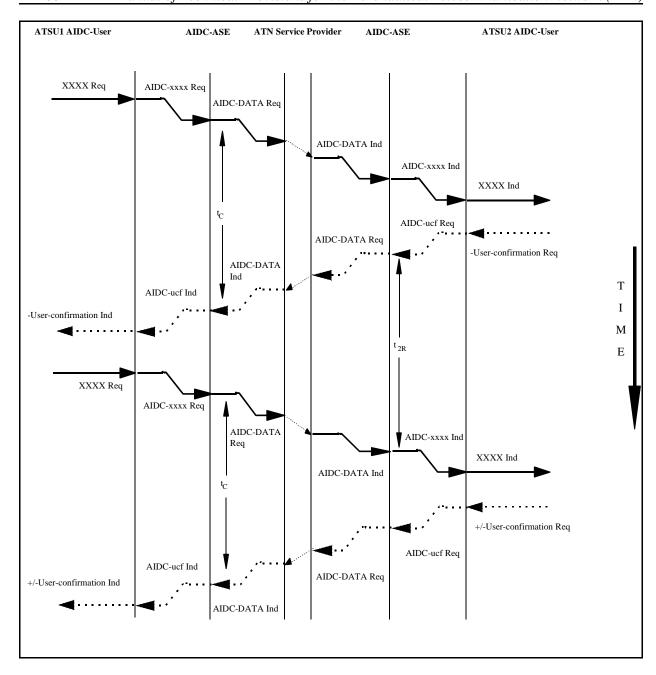
Figure 3.2.10-25: Sequence Diagram showing the sequence for a negative User Confirmation for all services except the Transfer-request, Transfer-conditions-proposal, Transfer-conditions-accept, and Info-Transfer services
