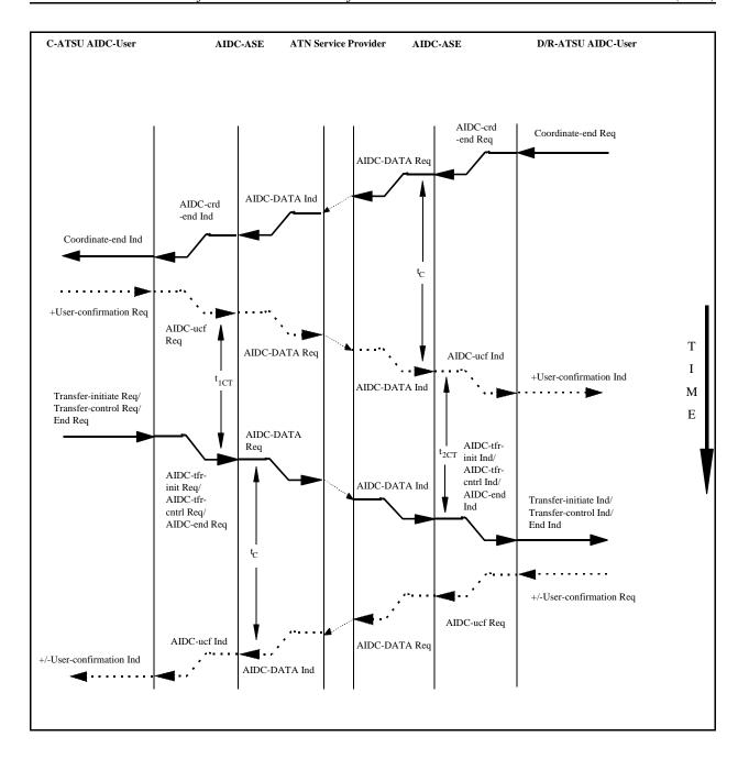
Figure 3.2.10-9: Sequence Diagram showing the start of the Transferring Regime through the invocation of the Transfer-initiate service
