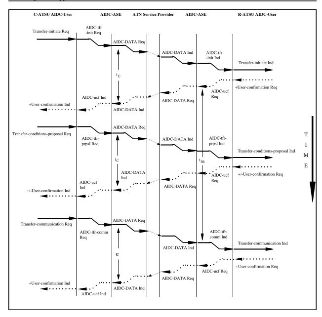
Figure 3.2.10-14: Sequence Diagram showing the invocation of the Transfer-conditions-proposal service, with predicate P1 false, followed by Transfer-communication service
