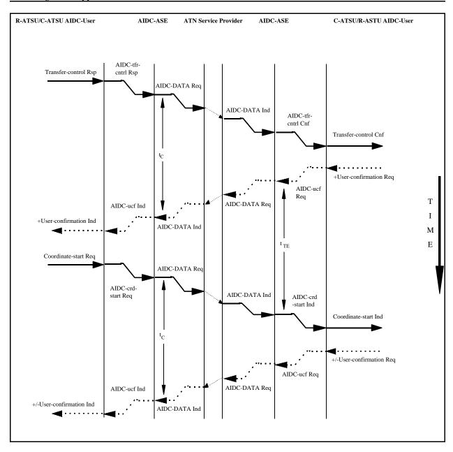
Figure 3.2.10-20: Sequence Diagram showing the re-entry into the Coordinating Regime, after the end of the Transferring Regime, through the invocation of the Coordinate-start service
