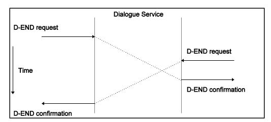
Figure 4.2-4. D-END collision sequence diagram (DS-User view)
