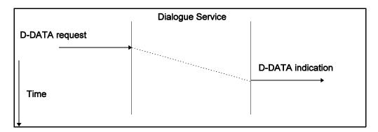
Figure 4.2-2. D-DATA sequence diagram
