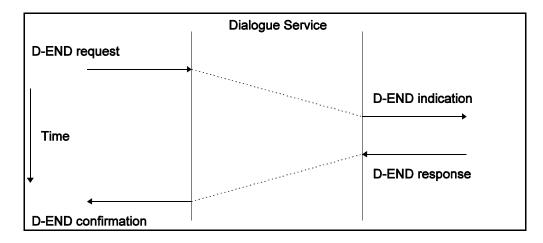
Figure 4.2-3. D-END sequence diagram
