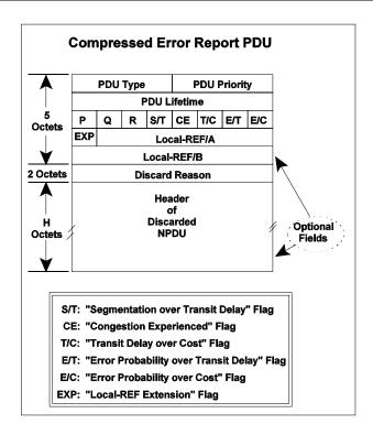
Figure 5.7-5 Compressed Error Report PDU
