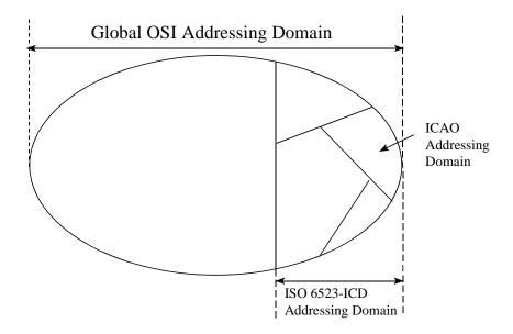
Figure 5.4-1 The Global OSI Network Addressing Domain
