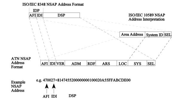
Figure 5.4-3 Derivation of the ATN NSAP Address Format
