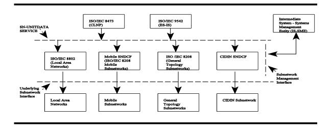
Figure 5.7-1 Relationship of SNDCFs to SN-Service and underlying Subnetworks
